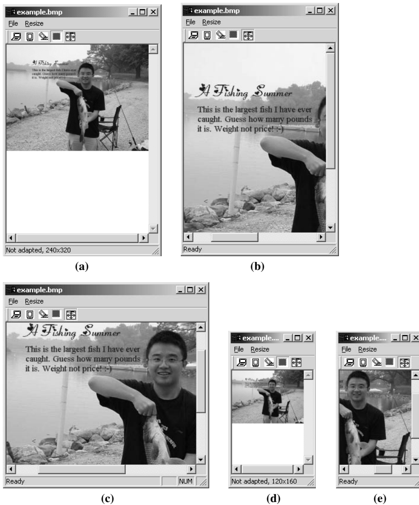
Fig. 11. An example comparing the proposed attention model with the conventional approaches to adapting images. a Direct down-sampling for pocket PC. b Attention-based method for pocket PC. c A better adapted result by rotation for pocket PC. d Direct down-sampling for Smartphone. e Attention-based method for Smartphone
